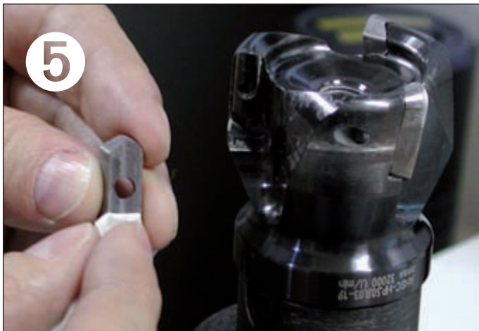
5 When indexing an insert to use the second edge, clean all location and support faces of the insert.
