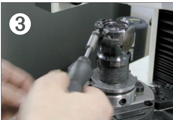
3 With the tool mounted in the presetting equipment or the assembly station, undo each insert screw and remove each insert.
