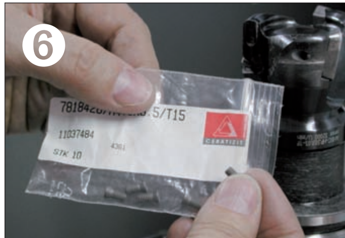
6 HSC machining: when mounting a new insert, always replace the old clamping screw with a NEW one.
