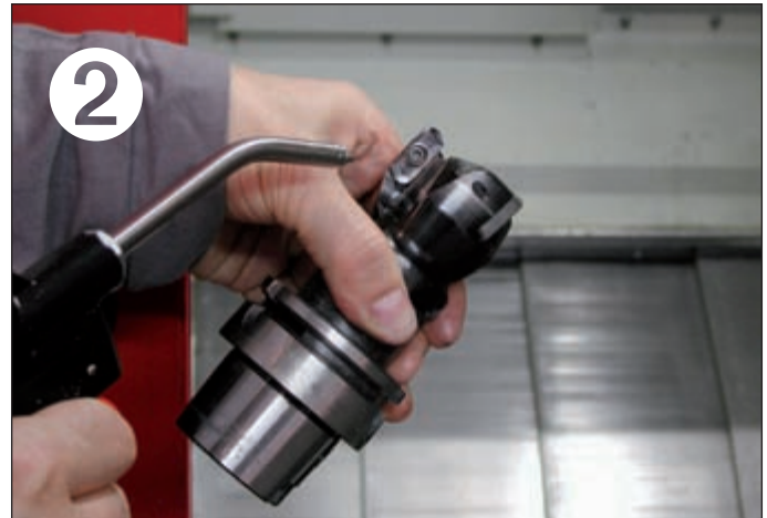
2 Clean with compressed air, taking care to protect eyes and exposed skin.
