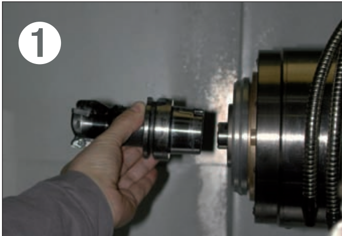
1 At the end of tool life remove the used tool from the machine spindle.
