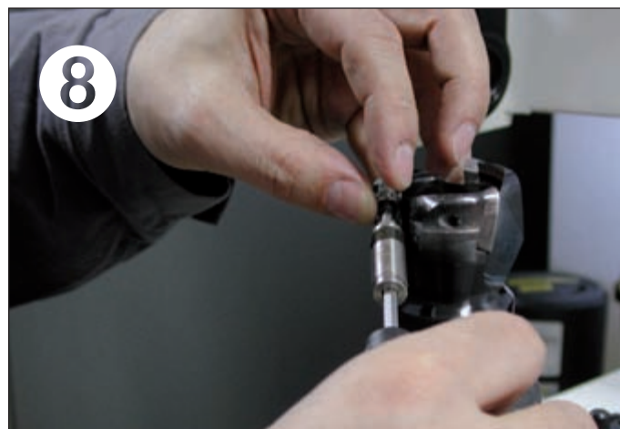
8 Keep pressing the insert onto the location faces while tightening the screw.
