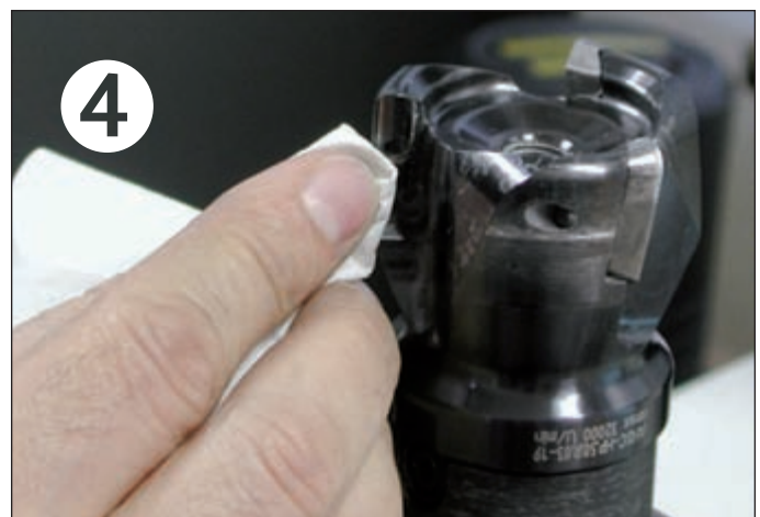
4 Clean the insert seat and check for damage.
