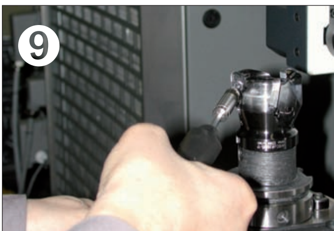
9 Clamp the insert using a preset torque key - see CERATIZIT literature for torque values. When reaching the torque setting the key clicks (do not attempt to tighten more than recommended torque values).
