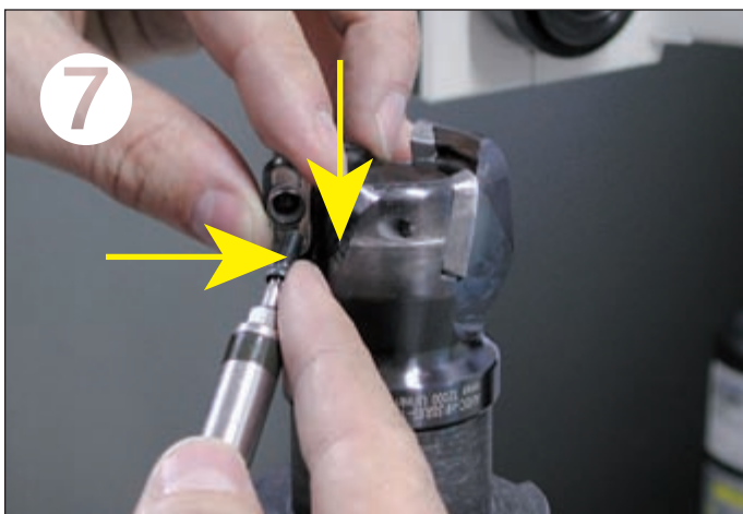
7 Place insert in cleaned pocket pressing it onto the location faces with two fingers.
